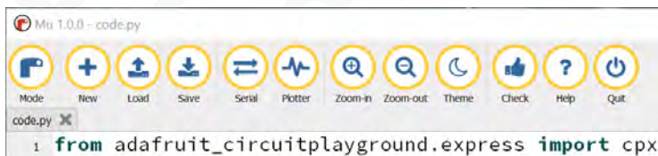
FIGURE 6-10. The Serial icon in the Mu editor, fifth from the left, has a double arrow icon.
